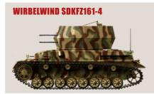
The Wirbelwind was a development of the Panzer IV designed to provide a vehicle offering AA fire support, armed with the standard 20mm AA qun quadruple mounting.
