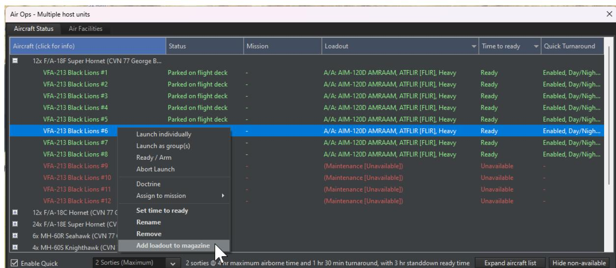
This makes it easy to populate the host platform's magazines with weapons compatible with the selected loadout, and thus quickly allocate sufficient weapons for this loadout.
